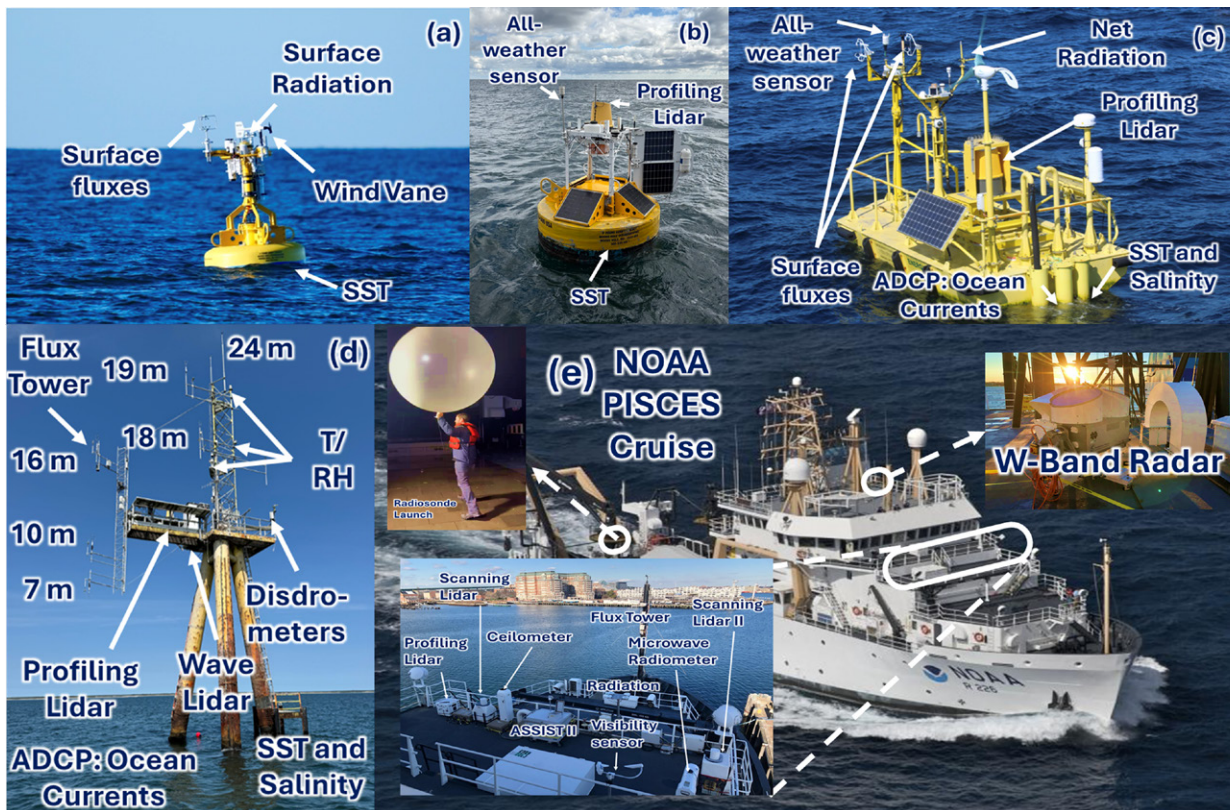
FIG. 5. WFIP3 offshore platforms and buoy systems, including (a) WHOI sentinel surface buoy, (b) WHOI lidar buoy, (c) DOE lidar buoy, (d) WHOI Air-Sea Interaction Tower (ASIT) and (e) NOAA PISCES winter cruise.
